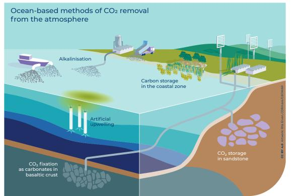
Figure 2: Illustration of ocean-based CDR processes that are being assessed within OceanNETs and CDRmare.
