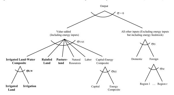
Figure A.1. Nested tree structure for industrial production process in GTAP-W (truncated)
