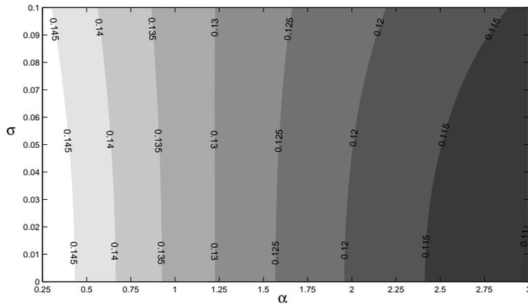
Figure 6: Optimal mitigation - Contour plot in the  $\alpha - \sigma$  space for high  $S$  and low  $K$ , i.e.  $(S,K)=(3500,500)$ .
